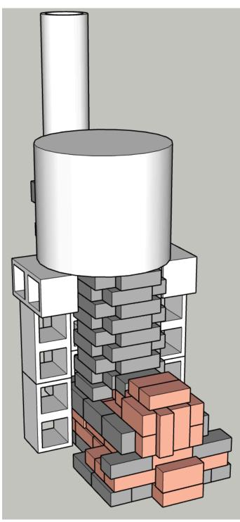
Hard bricks are placed over the firebox opening and the fuel (the skinnier the better) is fed in from the top. This creates a "self-feeding" fire that burns from the bottom up.
