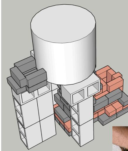
When placing the chimney bricks, snug them up agains the kiln body as best as possible and add worm band around the entire kiln and bricks to hold them in place.
