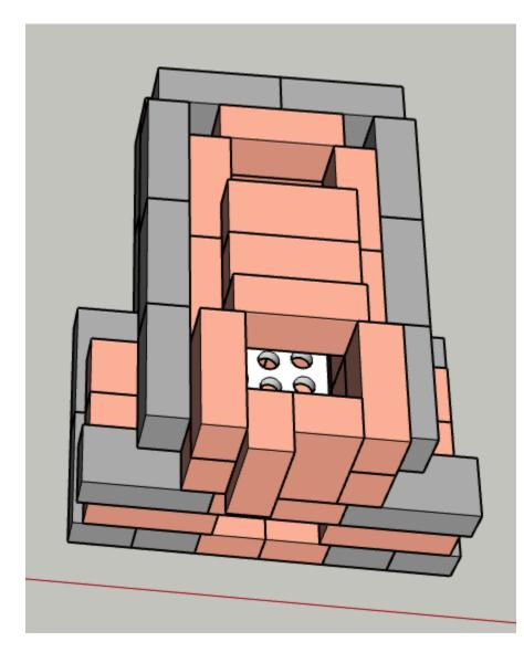
The 2 hard bricks covering the bottom of the J-Tube could be substituted with soft brick if you have extra soft brick.
