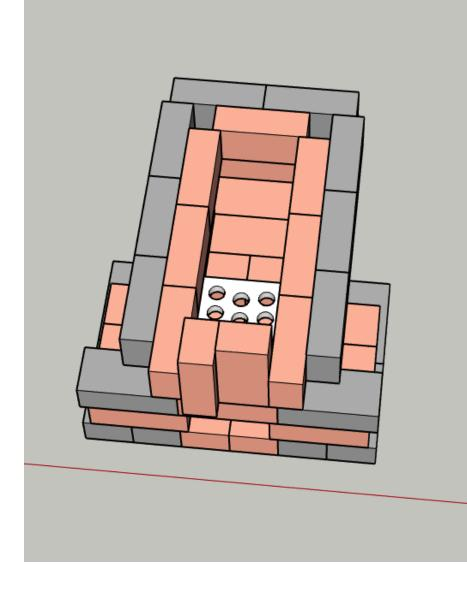
The void space in the back corners (bottom of heat riser), should be filled with kaowool or an insulating cobb/castable. If you have extra soft bricks you can cut some to fill in the spaces.
