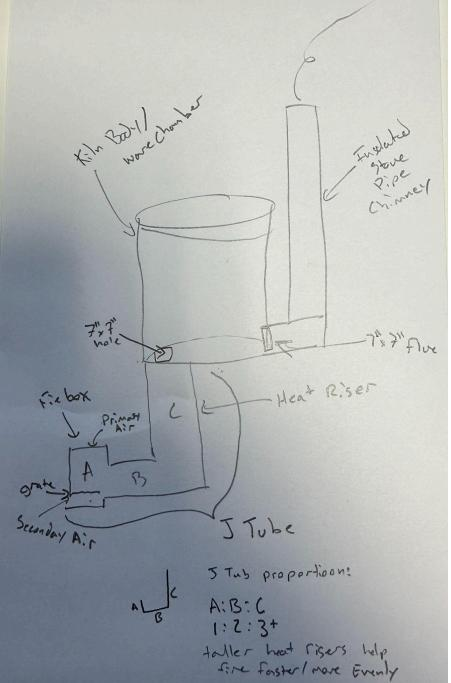
This diagram shows the rough layout and proportions of the parts of the rocket kiln. The proportions of the J tube, heat riser and flue openings are important for the efficient firing of a rocket kiln. This is designed to fire in neutral/oxidation.
