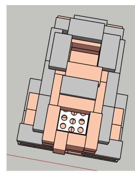
Here is an aerial view and side view of the added soft bricks to start the heat riser. The soft brick on top of the bottom of the J tube can be replaced with kaowool or insulating castable/cobb.
