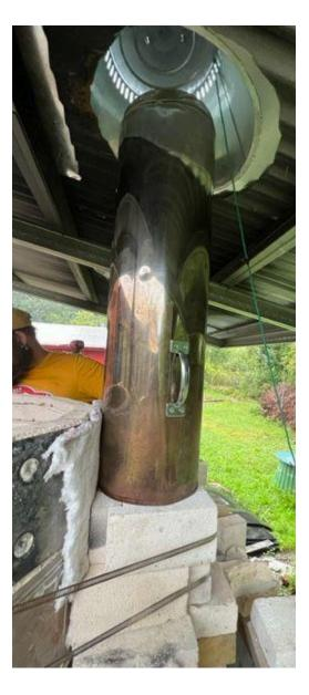
Here you can see the added 8" insulated stove pipe. We were able to fire to cone 10 in 3 hours with a 3' stove pipe. If you have a larger kiln body a 4' pipe or added brick layers may be necessary. This chimney could also be constructed from soft brick as the insulation increases the draw. If damper is present, band the chimney to the kiln so it will not be affected by wind.
