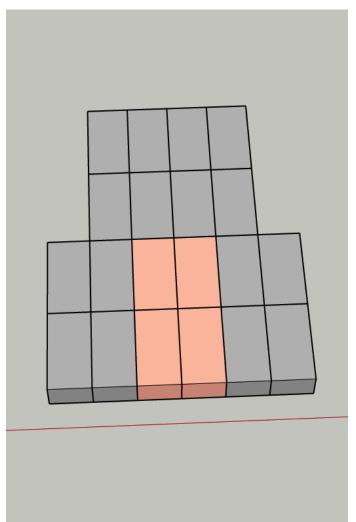
The hard bricks will be located underneath the firebox/grate.
