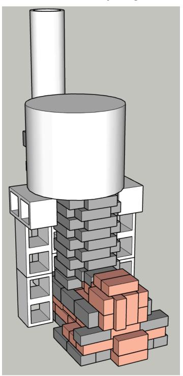
Hard bricks are placed over the firebox opening and the fuel (the skinnier the better) is fed in from the top. This creates a "self-feeding" fire that burns from the bottom.
