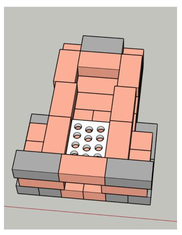
The grate should fit snug left to right. Make sure some air can move between the grate and J tube.
