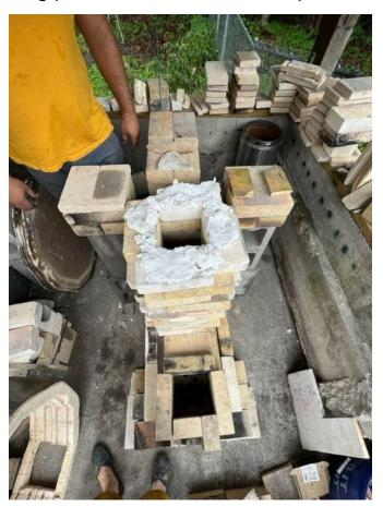
place the kiln bottom. Kaowool is used around the heat riser to form a gasket. If you are using refractory cobb/castable, this would be a good place to add some around the kaowool.
