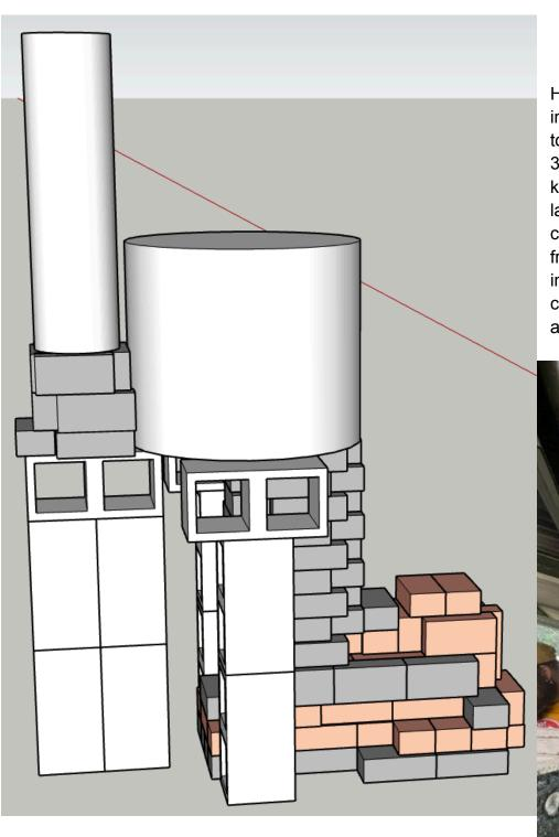
Here you can see the added 8" insulated stove pipe. We were able to fire to cone 10 in 3 hours with a 3' stove pipe. If you have a larger kiln body a 4' pipe or added brick layers may be necessary. This chimney could also be constructed from soft brick as the insulation increases the draw. Band the chimney to the kiln so it will not be affected by wind.
