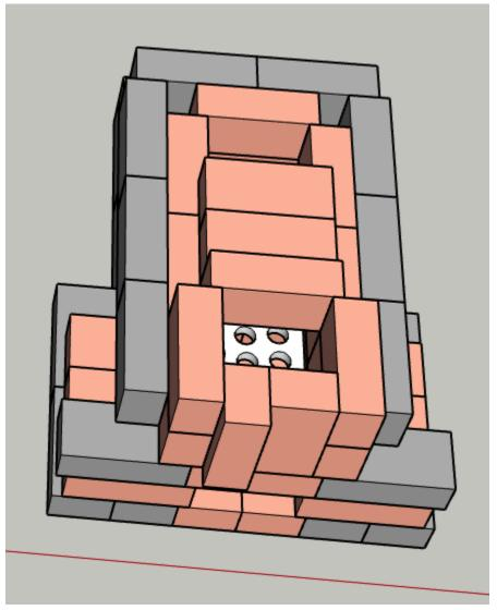
The top Layer of the firebox should be wrapped with a worm band to add strength to the upright bricks. When stoking, the wood will lean against the top edges and can force the bricks to separate if they are not braced. See below picture of worm banded firebox in use.
