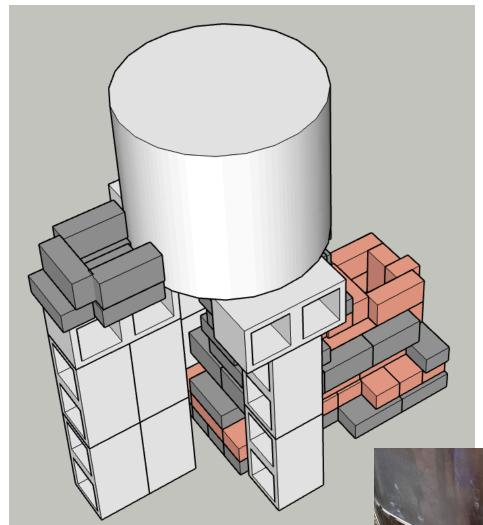
When placing the chimney bricks, snug them up agains the kiln body as best as possible and add worm band around the entire kiln and bricks to hold them in place.
