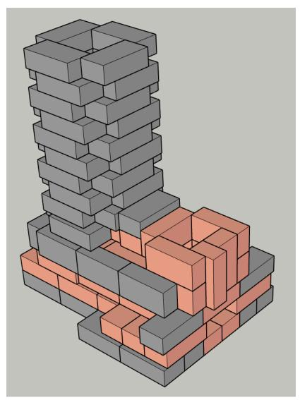
In this step you will finish building the heat riser. In this model, the heat riser has 10 total soft brick layers.
